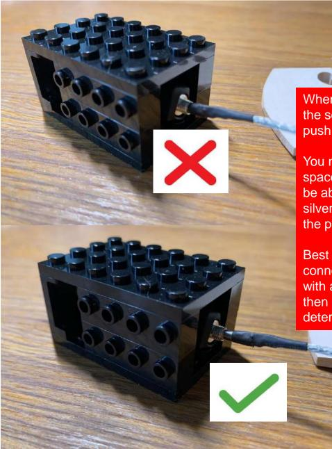
When connecting wire to the soundbox, DO NOT push the pin to the end,
