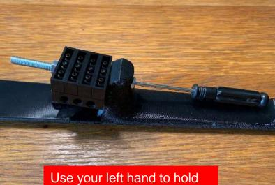
Use your left hand to hold the nut and screwdrive the screw very tight until the square block is firmly attached with violin neck.
