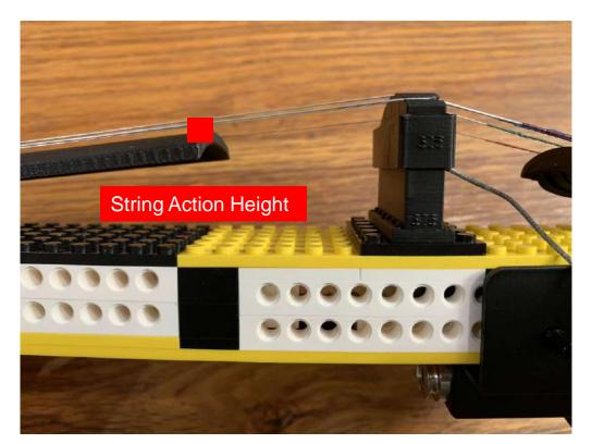
When strings are installed and after they are tuned properly, you may find string height to the fingerboard is too low or too high.
