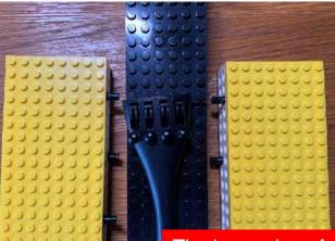
The long edge of sidebox interfacing with spine must be the smooth side.
